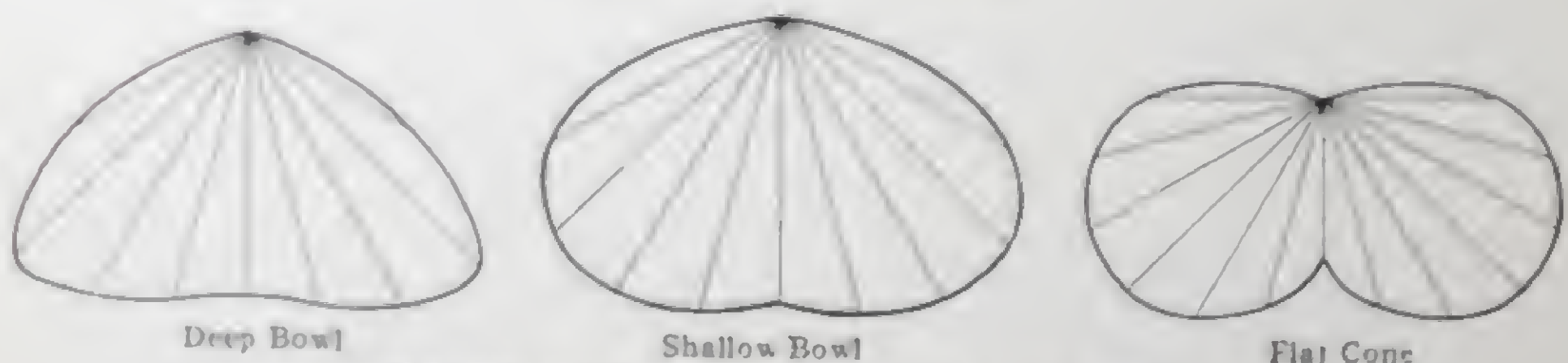
Distribution Curves of White Enameled Steel Reflectors
